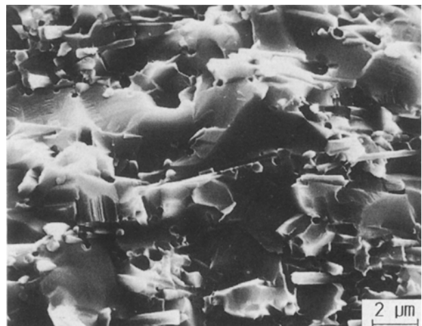
Figure 8 Extensive transgranular fracture of the alumina grains and pull-out of the SiC whiskers are observed on fracture surfaces produced at high crack velocities in the larger grained alumina reinforced with 20 vol% SiC whiskers, during static fatigue-crack growth.
